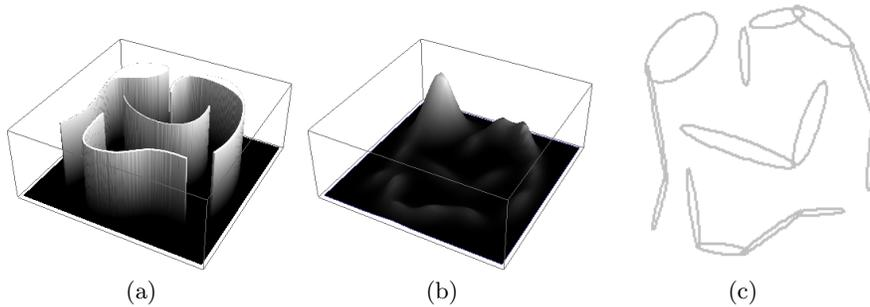
**Fig. 2.** CEC method applied to white regions of Fig. 3(a): (a) - uniform distribution, (b) - several Gaussian functions approximating given distribution, (c) - ellipses corresponding with those functions.
